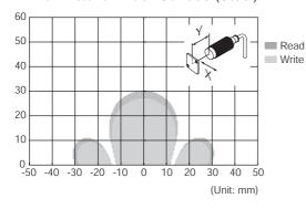
V680-HS63 and V680-D1KP66MT with Metal on Back Surface (Steel)
