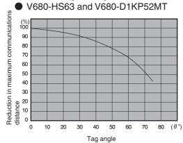
(Metal: Steel) Reduction in maximum communications (%) 100 90 80 70 60 50 40 30 distance 20
