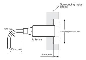
Do not bend the cable into a curve tighter than 22 mm in radius.
