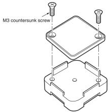
Install so that the mounting holes are aligned.
