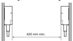
• Installing the Antennas in Parallel
