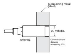
If the metal around the Antenna reaches the coil surface, the communications distance will be reduced significantly compared with mounting to a non-metallic surface.
