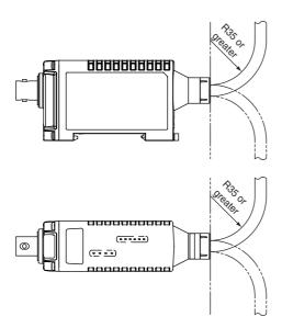
Do not bend the cable past a bending radius of 35 mm.
